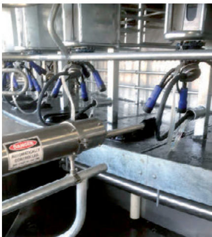
The auto teat spray system is controlled from the ID system, but it can stand alone.
