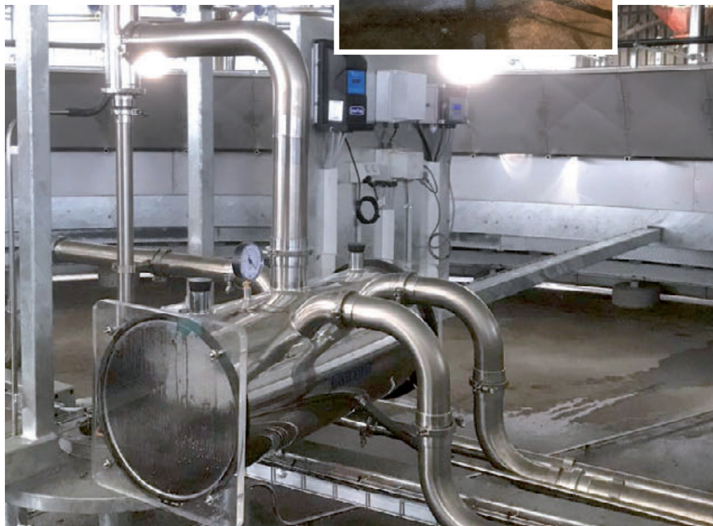
The sanitary strap includes stainless steel welded fittings for longevity. All the controls and power supplies are mounted on a single, easily accessible panel.
