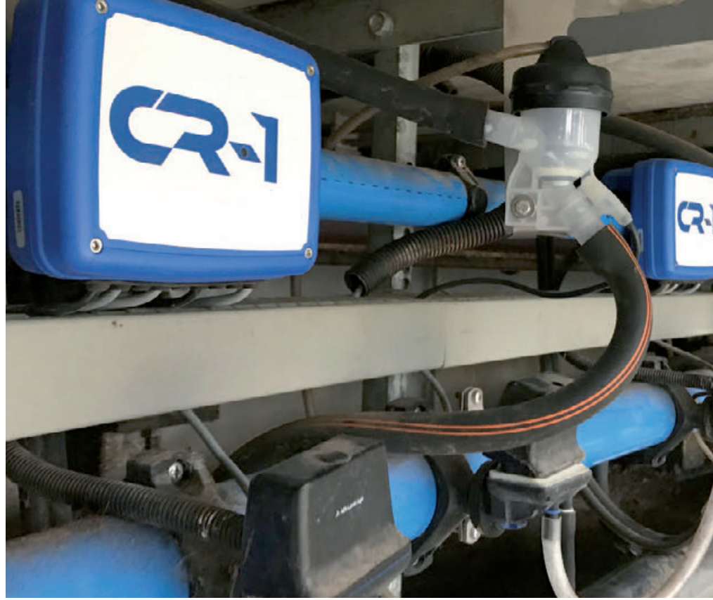
The CR-1 control boxes can be retro-fitted on an existing system which may be aging, allowing for the addition of the new wi-fi functionality.
