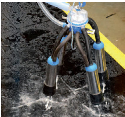
A cluster cleanse system back-flushes with a sanitiser and compressed air after every cow is milked.
