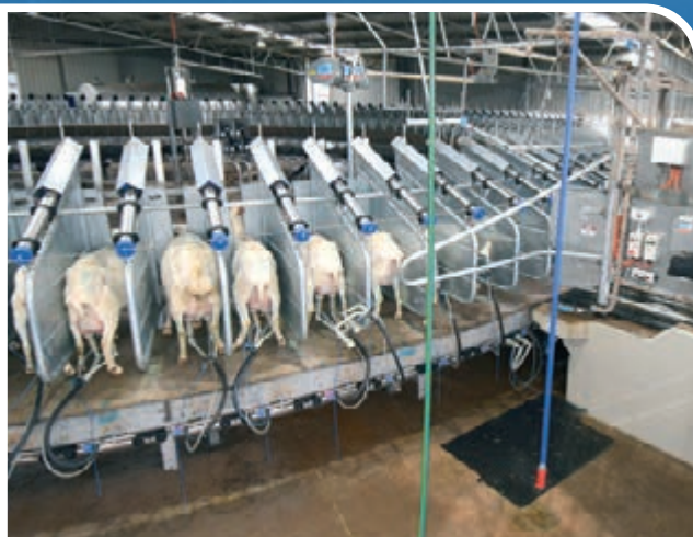
Daviesway successfully took on a technical project when it converted a 60-stand dairy cow rotary into a 120-stand goat dairy capable of milking 8000 goats in South-Western Victoria.
