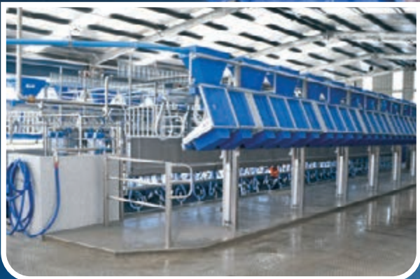
Rapid release configurations are an efficient take on the herringbone dairy when there is enough space.
